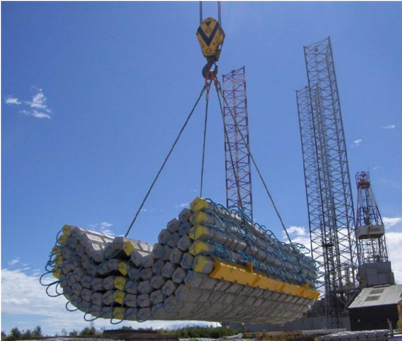
Figure 5.4.2: Speedloader lifting frame 21
