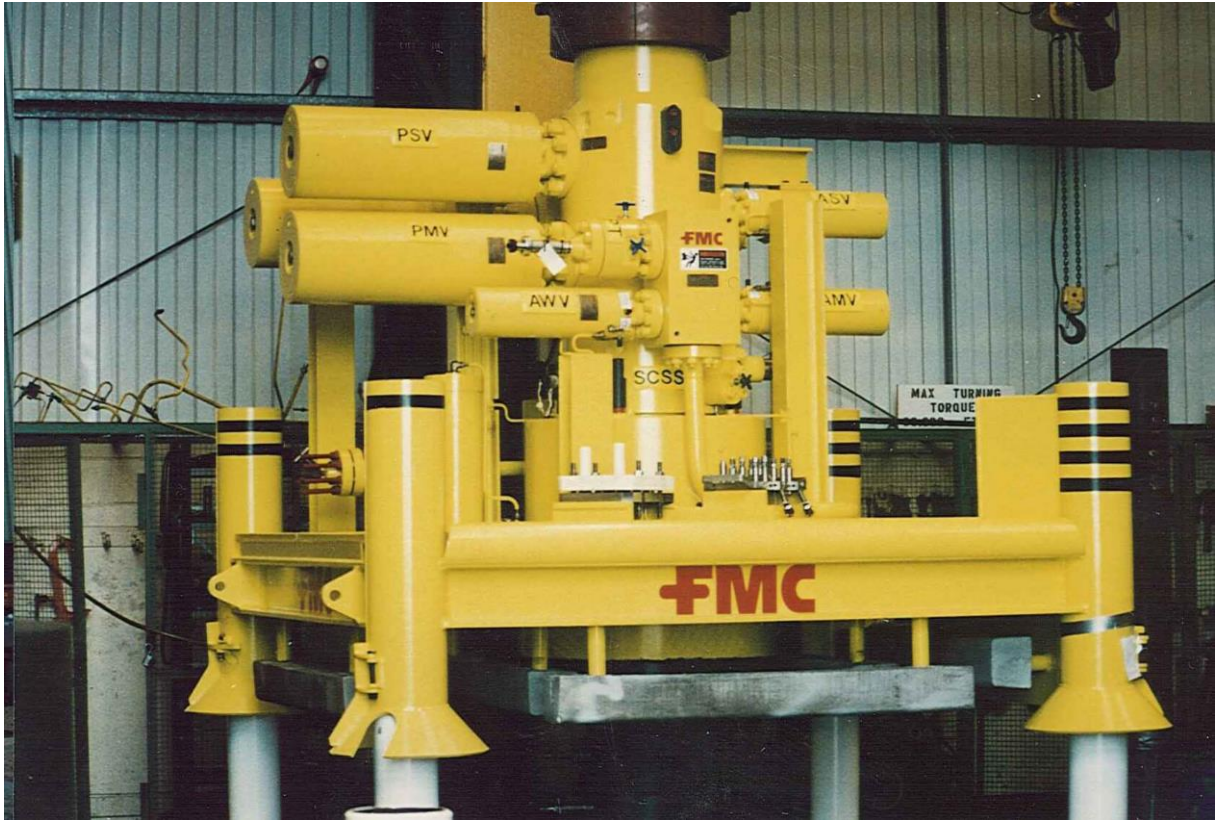
Figure 2.2.1 Photograph of subsea Xmas tree, Callisto ZM
